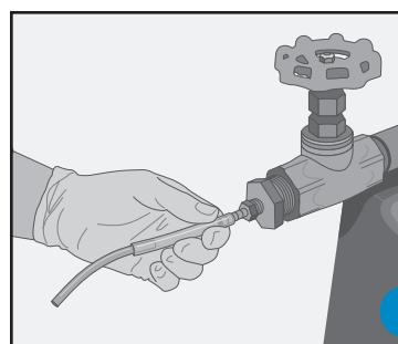
**6** **Flush the valve** as follows: 50 oz. for a 1" valve. 60 oz. for a 2" valve. (Tubing here is optional.)
