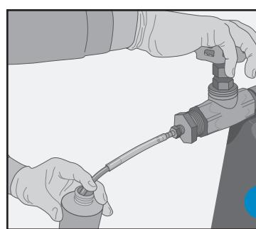
**7** **Fill the plastic bottle** 2/3 full. Shake the bottle. Discard the liquid. Fill the bottle to the neck and secure the cap tightly.
