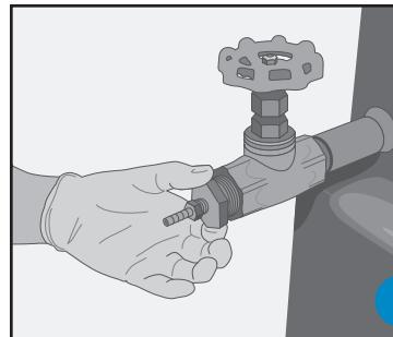
**5** **Affix the tubing reducer** to the inside of the clean valve fitting. Tighten with moderate torque.
