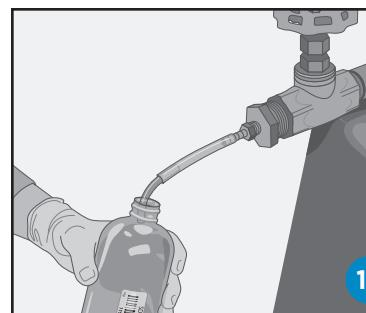
**12** **Draw 50 ml of liquid** into the sampling syringe and evacuate the syringe. **Draw another 50 ml of liquid** into the syringe.
