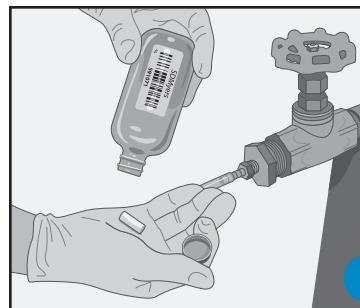
**8** **Remove and discard the desiccant tablet** from the glass bottle. (This is an **extremely important** step.)
