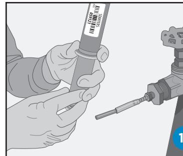
**10** **Fill the small glass bottle** to the very top. Ensure bottle is **full to the extreme top** of the bottle, and secure the cap very tightly.
