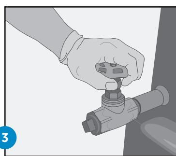
**3** Verify that **the valve is shut off** before removing the front plug.
