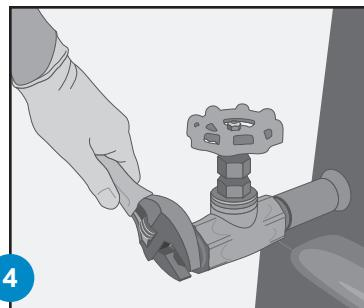
**4** **Remove the front plug** and inspect for debris. Wipe the inside of the valve fitting with a clean cloth.
