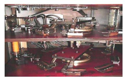
coating is generally very dark and is often mistaken as a carbon deposit or as evidence of coking. The photo below shows deposits of filming compounds on the contacts of an LTC. The smooth appearance is unlike the typical pebbly surface of a coke deposit after it forms in an electrical device. Notice also those surfaces of the contacts that have been wiped clean and show up as bright areas of relatively clean conductor.
